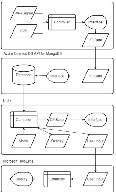
Figure 1: System Architecture
