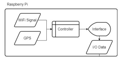
Figure 2: Raspberry Pi data flow
