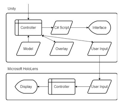
Figure 4: Data flow from Unity into the Microsoft HoloLens
