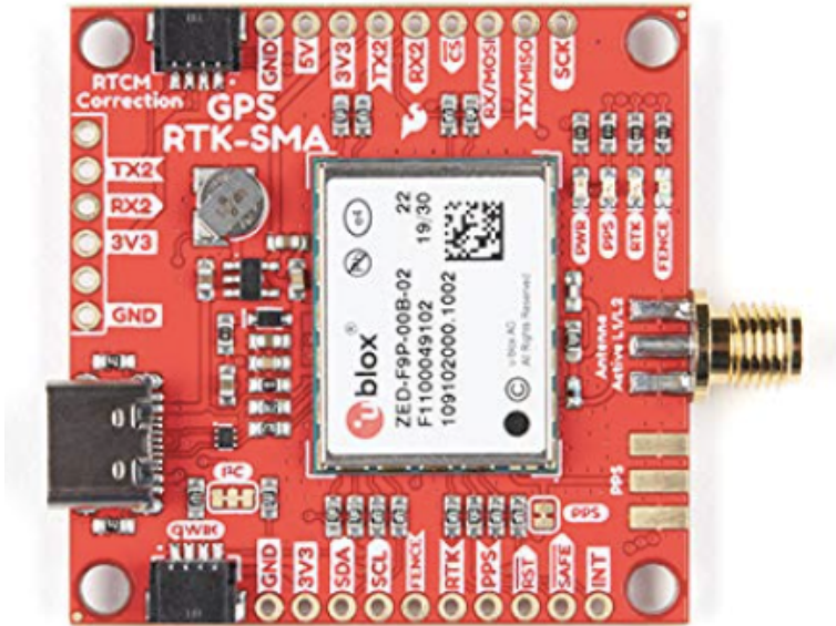
Figure 8: Antenna: ZED F9P RTK BOARD
